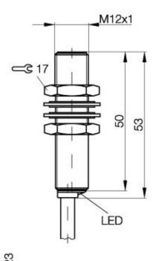
Inductive Sensors BES M12MI-NSC40B-BP03 M12x1 x 53 normally-open Sn=4mm shielded
